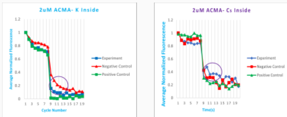
Figure 6: NavAb K-conductivity is stronger than Cs-conductivity as indicated by the initial affinity table
